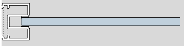
Deubl PT 35 frame profile with glass penetration
